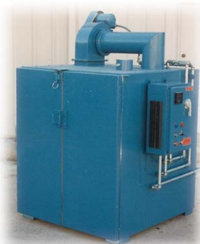
This walk-in oven measuring 6 ft. wide x 6 ft. long x 6 ft. high reaches temperatures of 600° F. with 60 kW of electric power. The recirculating ductwork on the top was unique to this application.
