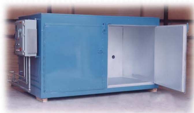
This natural convection type walk-in oven provided adequate temperature without the use of a recirculating blower. Special care was given to the layout of the heating system.
