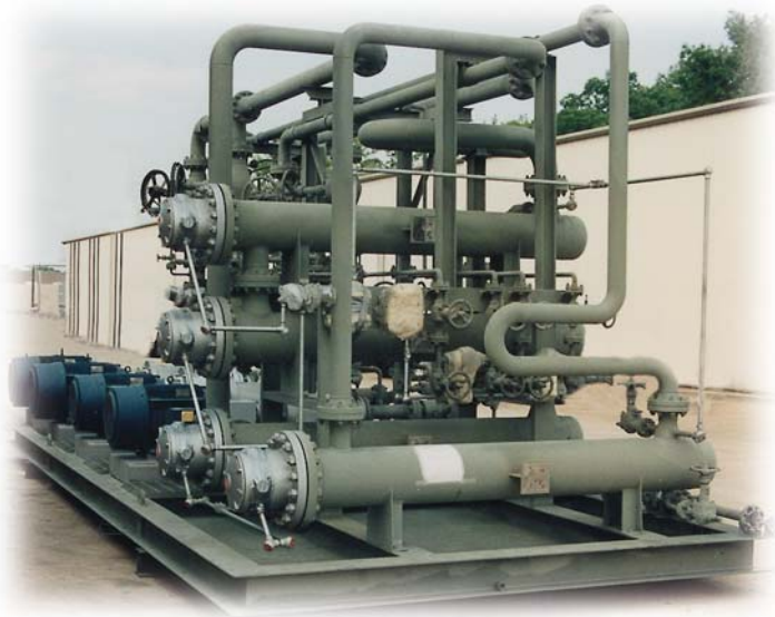
800 kW dual zone Hot Oil System designed for Class I, Group D hazardous location. Unit included spare magnetic drive pumps, special thermal expansion loops, and customer specified paint.
