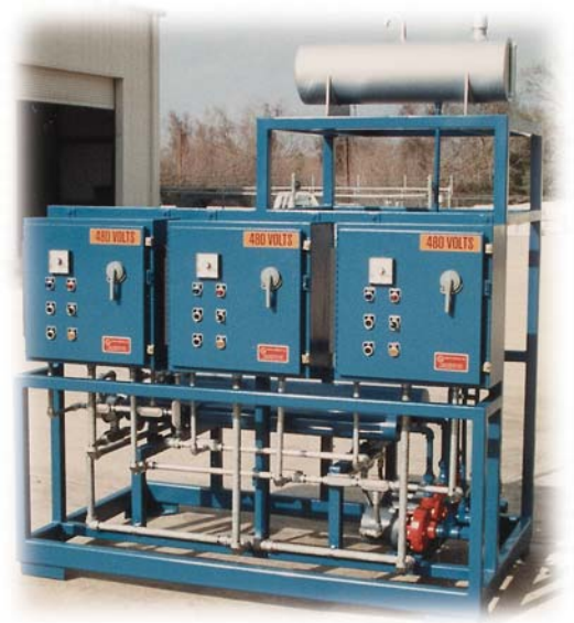
Triple zone Liquid Heating System mounted on a single frame with a common expansion tank.
