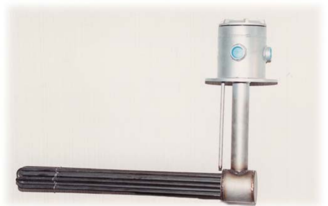
Type LH (horizontal) over-the-side heater with integral cover plate. Also available, Type LV (vertical) which has a vertical mounted heater bundle. Heater assembly available with bundle sizes as large as 8 inches in diameter and lengths to 165 inches as standard.
