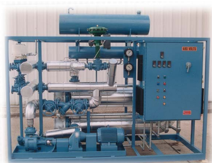
Modified GHOS Hot Oil Systems provided multi-zoned heating to the customer's process.
