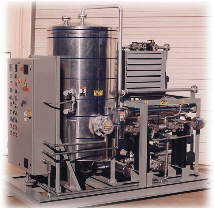
Electric Heating / Air Cooling package with reservoir tank. Transmission fluid heating system for preheating fluid prior to transmission testing. System included cooler package for full temperature control.
