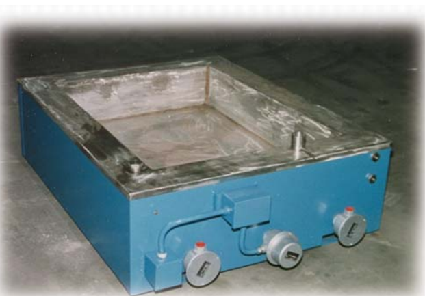
Rectangular Hot Melt Tank with “double tank” construction and a special heat transfer liquid in the outer tank which allows temperature control to \pm 2 degrees.
