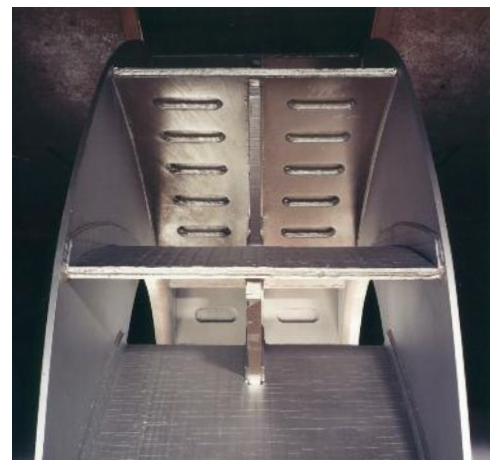
Top: Manufacturing of centrifugal fan impellers Above: Detail showing wear plate fittings
